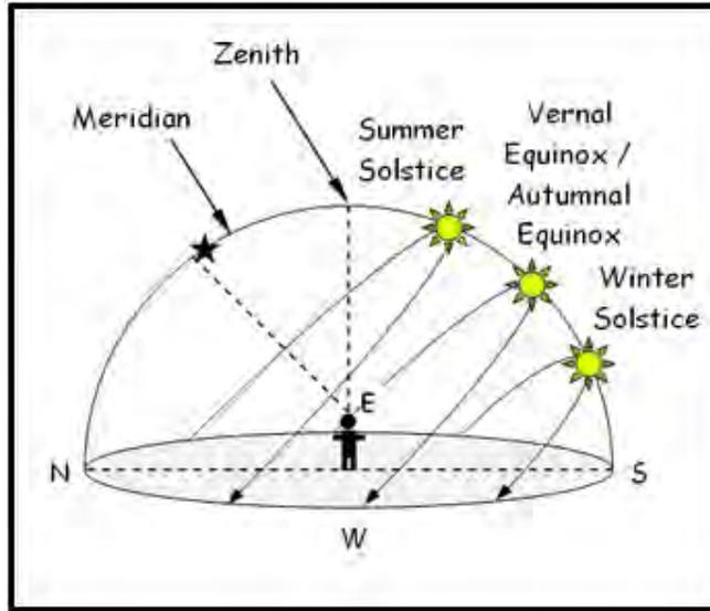
1.2.12 When the sun is at an angle of greater than 90 degrees from north in an easterly direction and an angle of greater than 90 degrees from north in a westerly direction any reflection from the solar panels is at an angle above the horizontal.
